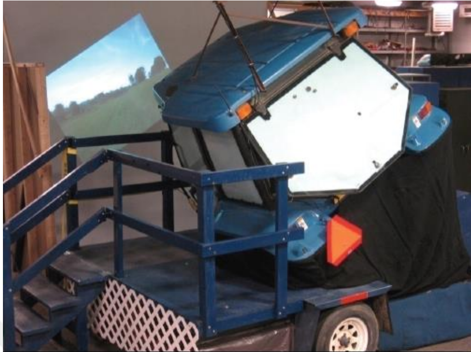
Figure 6 An example of tractor cab roll simulator, with simulator tilted to 30°. [23]
