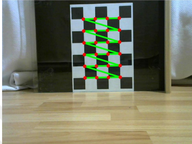
Figure 21 Detected corner points in camera calibration
