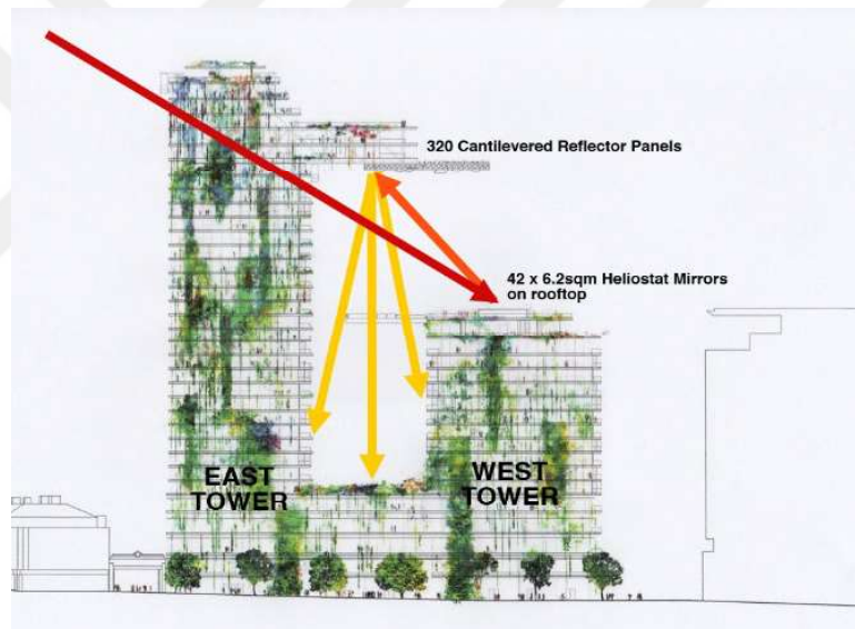
Figure 82. The Working System of Heliostat Application. (Url 70)
