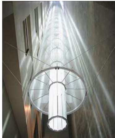
Figure 38. Solar Light Pipe Application. (Url 32)
