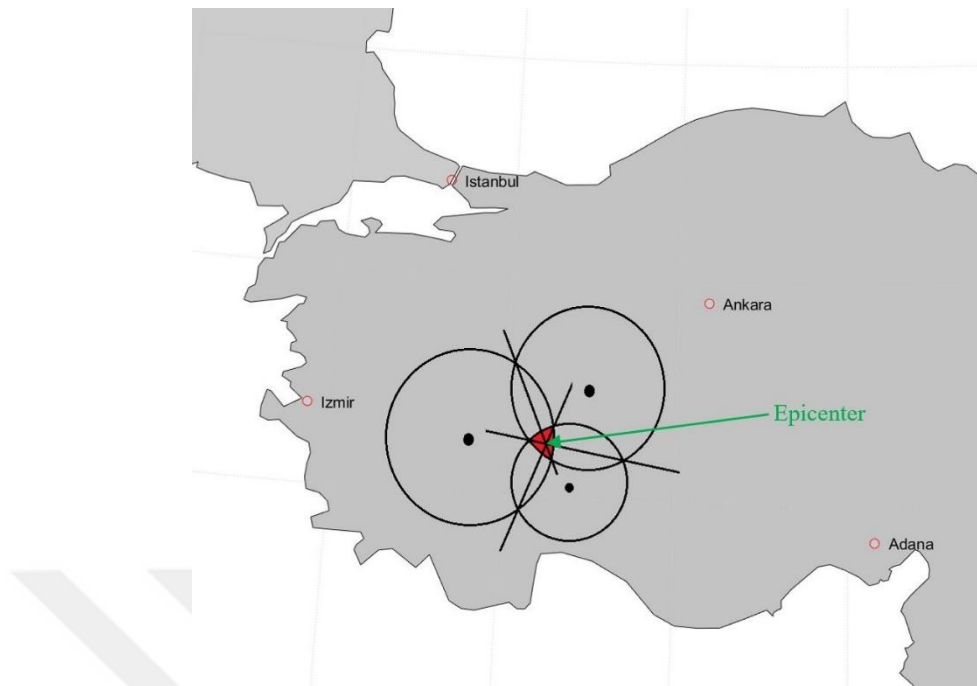
Figure 1.1: A process called triangulation uses seismic data from three locations to identify the epicenter of an earthquake.
