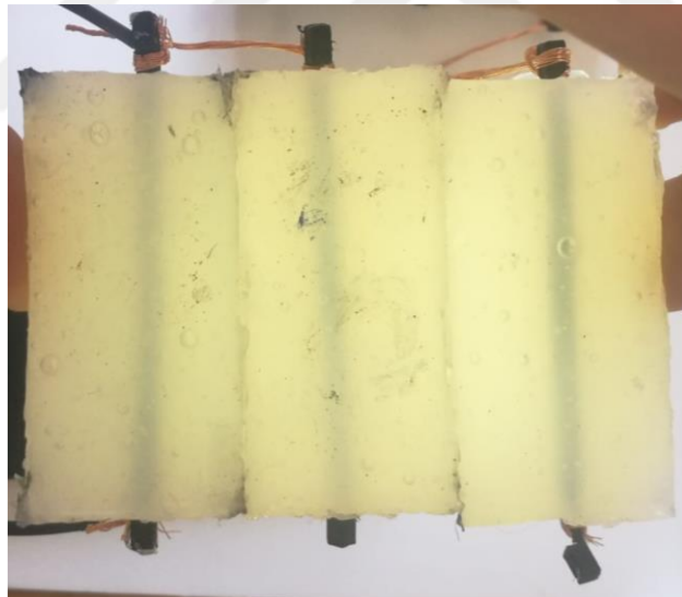
Figure 2.8: Prepared Straight Line Shape Conductive Layer Test Specimens.
