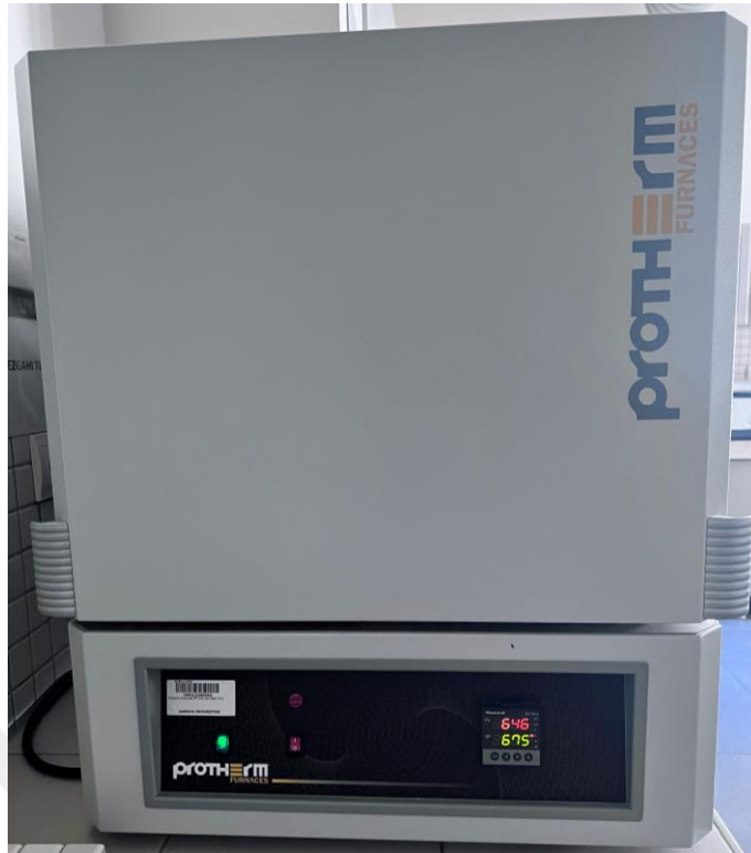
Figure 2.2: Protherm Furnaces P1 115M heat treatment furnace.
