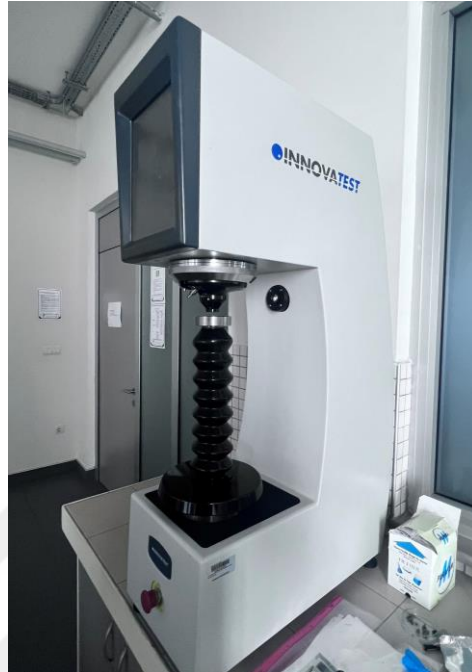
Figure 2.6: INNOVATEST Nexus 7500TM Universal Hardness Tester.
