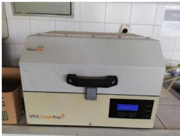
Figure 2.3: SPEX SamplePrep 8000M Mixer/Mill ball milling device.
