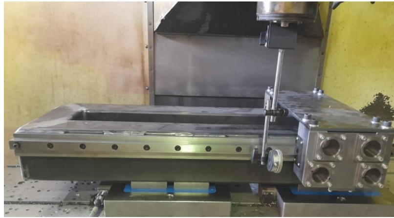
Figure 4.2.1: LR Lateral Run-Out Test With No Load
