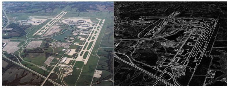
Figure 51 Example of Sobel edge detection
