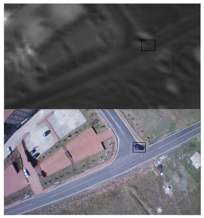
Figure 61 Example of normalized squared difference application
