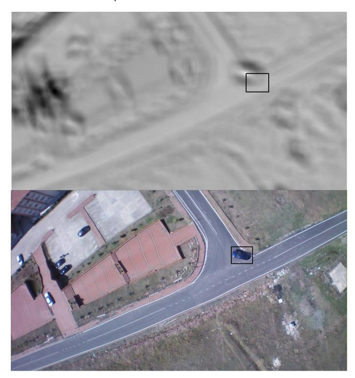
Figure 63 Example of normalized cross-correlation application
