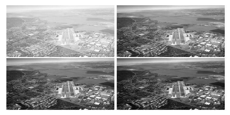
**Figure 41** Example of power-law function application: a) original aerial image, b) result when y=3.0, c) result when y=4.0, d) result when y=5.0, for all c=1
