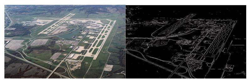
Figure 52 Example of Prewitt edge detection
