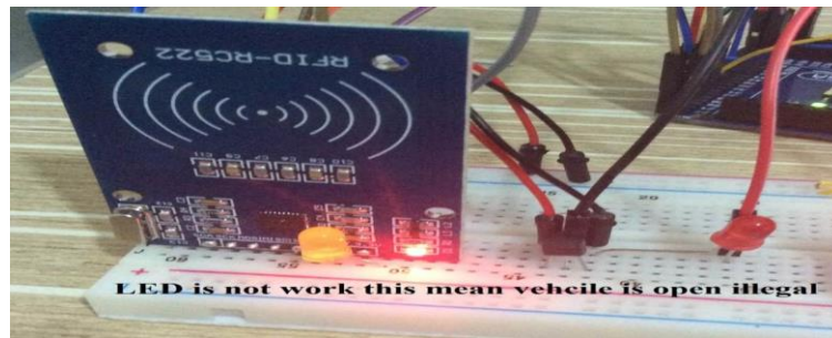
Figure 22: RFID reader recognize the door open illegally
