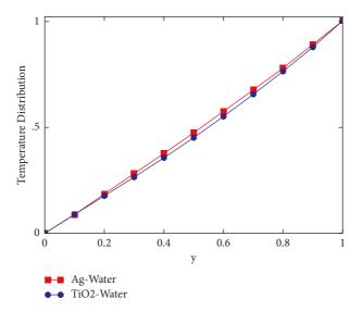
FIGURE 7: Correlation among nanofluids for temperature, when t = 3,  $\alpha = 0.2$ , Q = 3, and Pr = 6.2.
