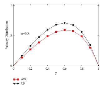
FIGURE 2: Correlation between the velocities through CF [37] and present, when Pr = 6.2, t = 3, M = 0.2, Gr = 20, Q = 0.5,  $\phi_{hnf} = 0.08$  and  $\beta = 0.8$ .
