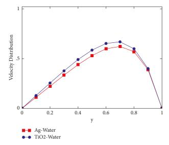
FIGURE 6: Correlation between nanofluid for velocity, when Pr = 6.2, t = 0.4, Gr = 40, Q = 0.5, M = 10,  $\beta = 2$  and  $\alpha = 0.2$ .
