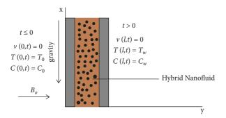
FIGURE 1: Formation of microchannel and coordinate system.
