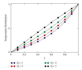
FIGURE 9: Effect of heat source Q on temperature when Pr = 6.2, t = 0.4,  $\phi_{hnf} = 0.2$  and  $\alpha = 0.5$ .
