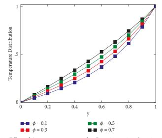
FIGURE 11: Effect of  $\phi_{hnf}$  on temperature after Pr = 6.2, t = 0.4, Q = 1.2 and  $\alpha = 0.5$ .
