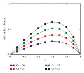
FIGURE 16: The influence of Gron velocity when  $\beta = 0, t = 3, Pr = 6.2, Q = 0.5, M = 4, \phi_{hnf} = 0.08, \beta = 0.2$  and  $\alpha = 0.5$ .
