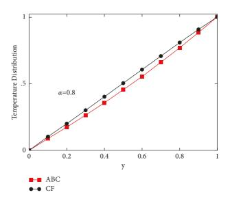
FIGURE 5: Correlation between the temperatures through CF [37] and ABC, Pr = 6.2, when t = 3, Q = 0.5 and  $\phi_{hnf} = 0.04$ .
