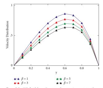
FIGURE 14: The velocity effect of the BT fluid *beta*, Pr = 6.2, Gr = 30,  $\phi_{hnf} = 0.08$  when t = 3, Q = 0.5, and  $\alpha = 0.5$ .
