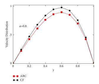
FIGURE 4: Correlation between the velocities through CF [37] and ABC, Pr = 6.2, when t=2, Q=0.5, Gr = 23, M=0.2,  $\beta = 0.8$  and  $\phi_{hnf} = 0.08$ .
