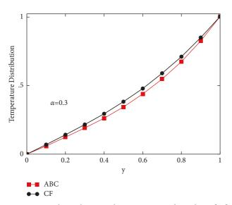
FIGURE 3: Correlation between the temperatures through CF [37] and present, Pr = 6.2, when t = 2, Q = 1.2 and  $\phi_{hnf} = 0.2$ .
