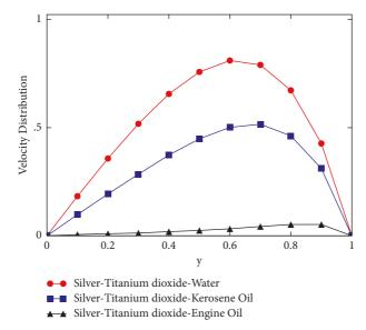
FIGURE 12: Comparison among base fluids (engine oil, water and kerosene) for velocity after Q = 0.5, t = 4, Gr = 30, M = 4,  $\beta = 0.2 \alpha = 0.5$  and  $\phi_{hnf} = 0.08$ .
