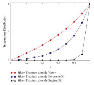
FIGURE 13: Comparison among unlike base fluids (engine oil, water and kerosene) for Temperature after  $\alpha = 0.5$ , t = 0.4, Q = 3 and  $\phi_{hnf} = 0.2$ .
