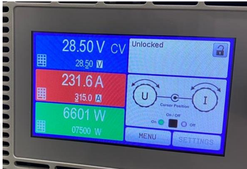
Figure 38: Power Supply Current Consumption
