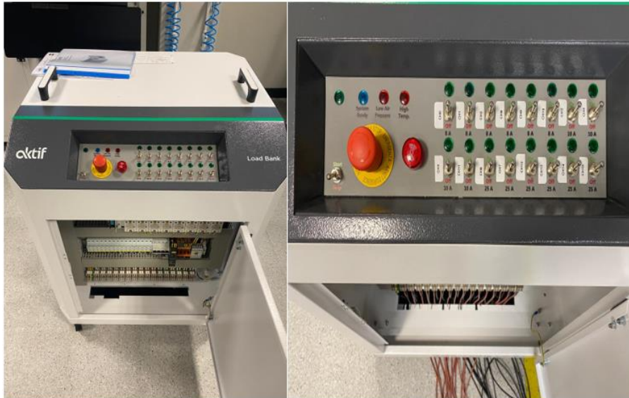
Figure 36: Resistive Load Bank
