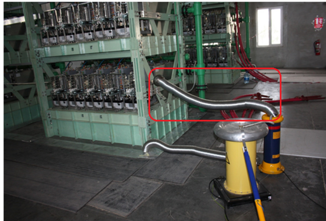
Figure 9. Aluminum flexible pipe for test cable shielding.
