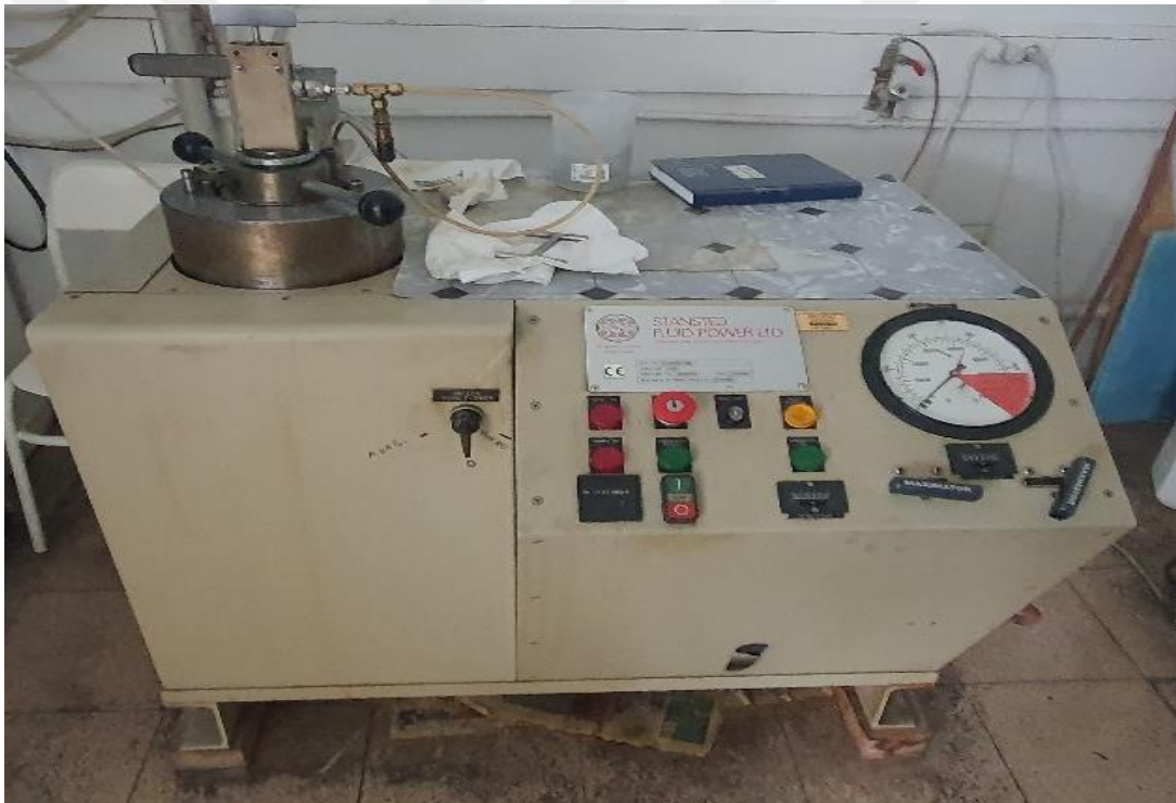
Figure 51: Cold Isostatic Press (CIP).
