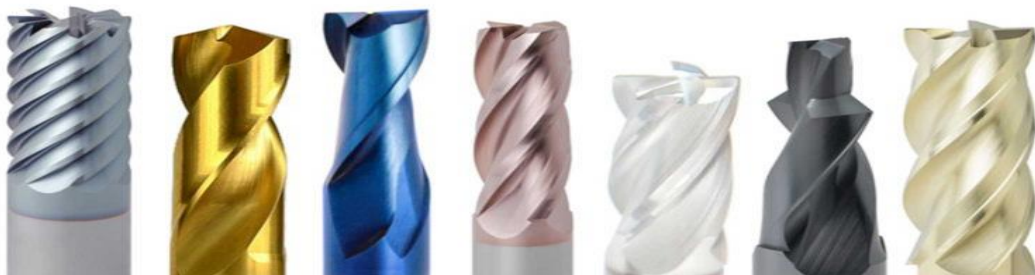
Figure 36: Physical Vapor Deposition PVD [86] [87].
