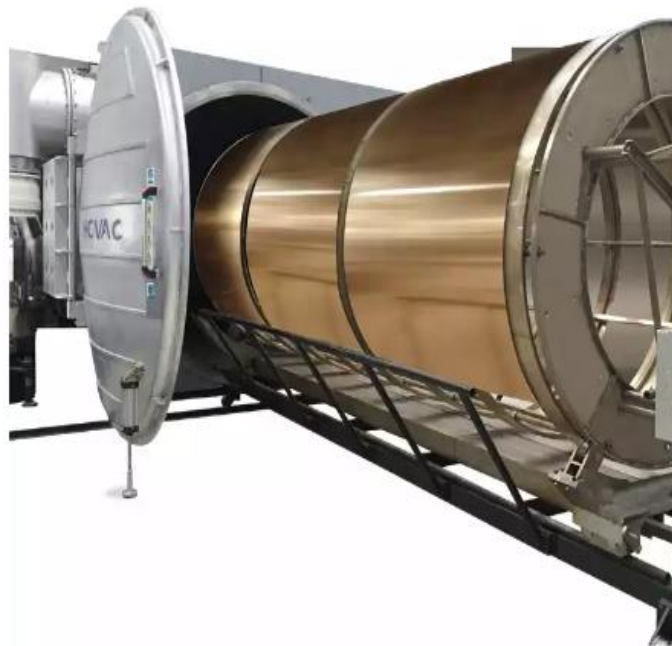
Figure 39: Plasma Spray Based – PVD (PS -PVD) [95] [96].
