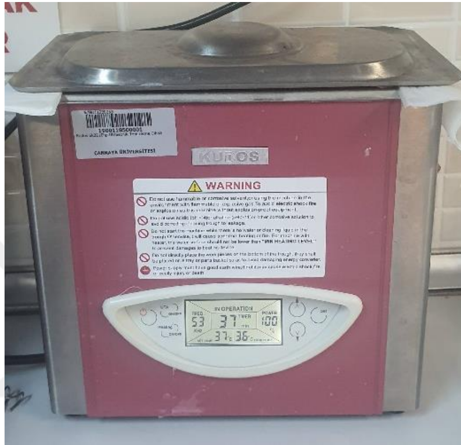
Figure 60: Ultrasonic cleaner, used for keeping the water hence the samples, at a constant temperature
